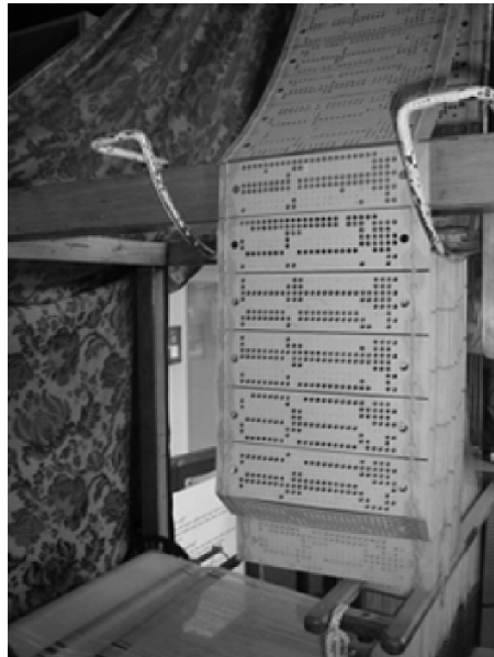
Figure 3.3: Punched cards controlling a mechanical loom (source: wikipedia)
